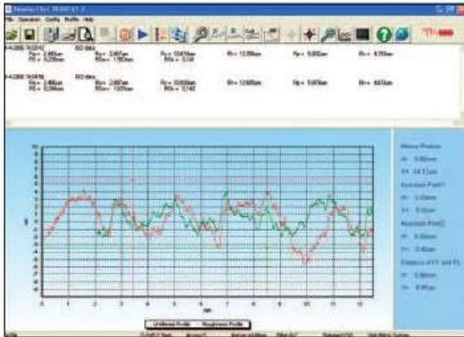
Profile display with roughness parameters in the program TimeSurf
